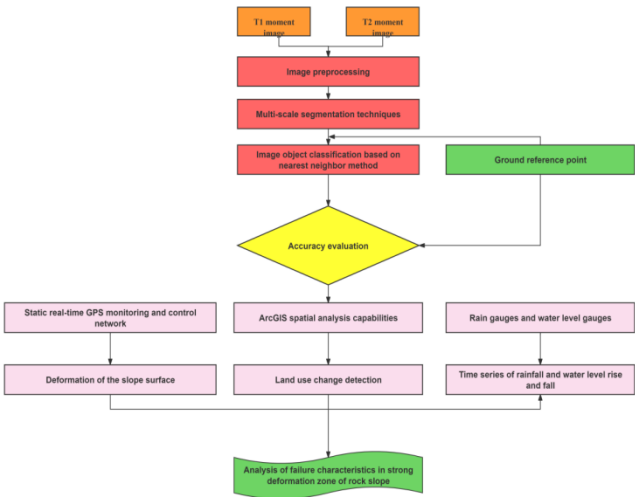
Figure 6. Landslide failure characteristics analysing based on “3S+AI”.
