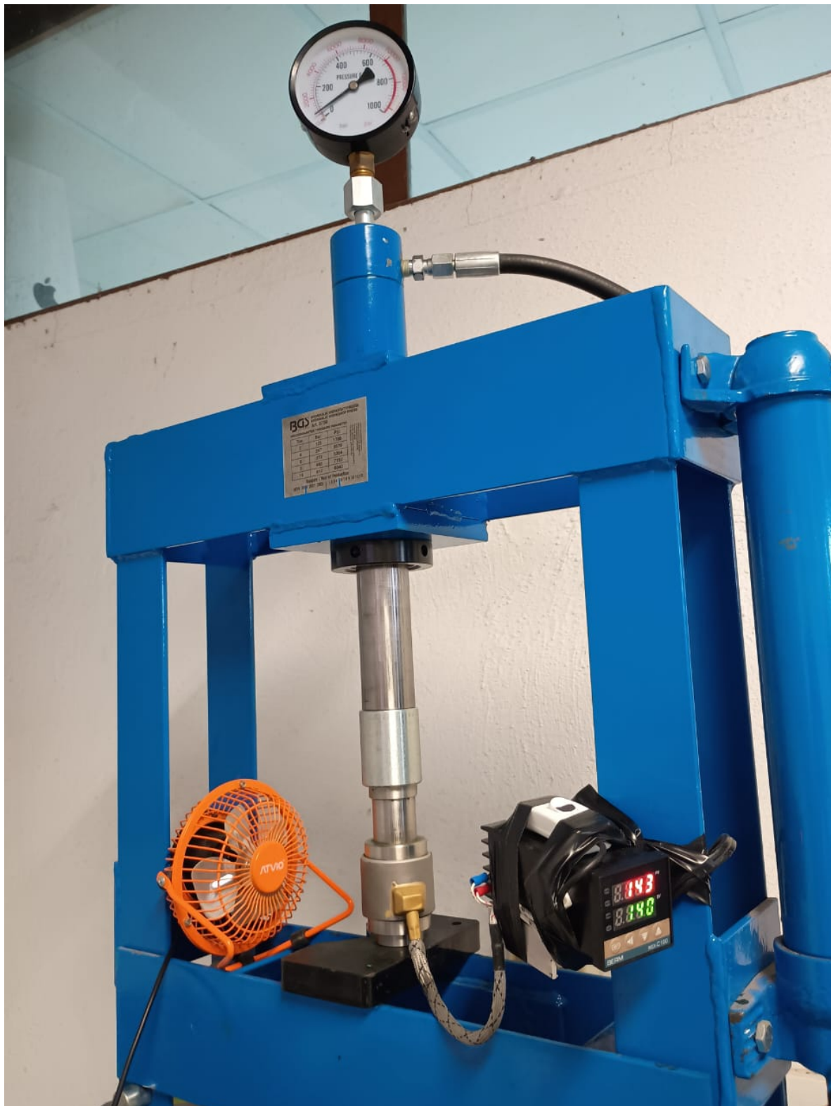
Figure 7. Metallography specimen mounting device placed in a hydraulic press.
