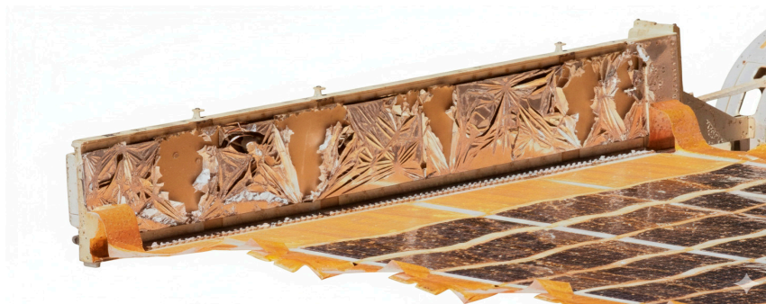
Figure 3. Damage to an ISS solar array blanket box caused by atomic oxygen exposure (Adapted from Holmes et al., 2023).
