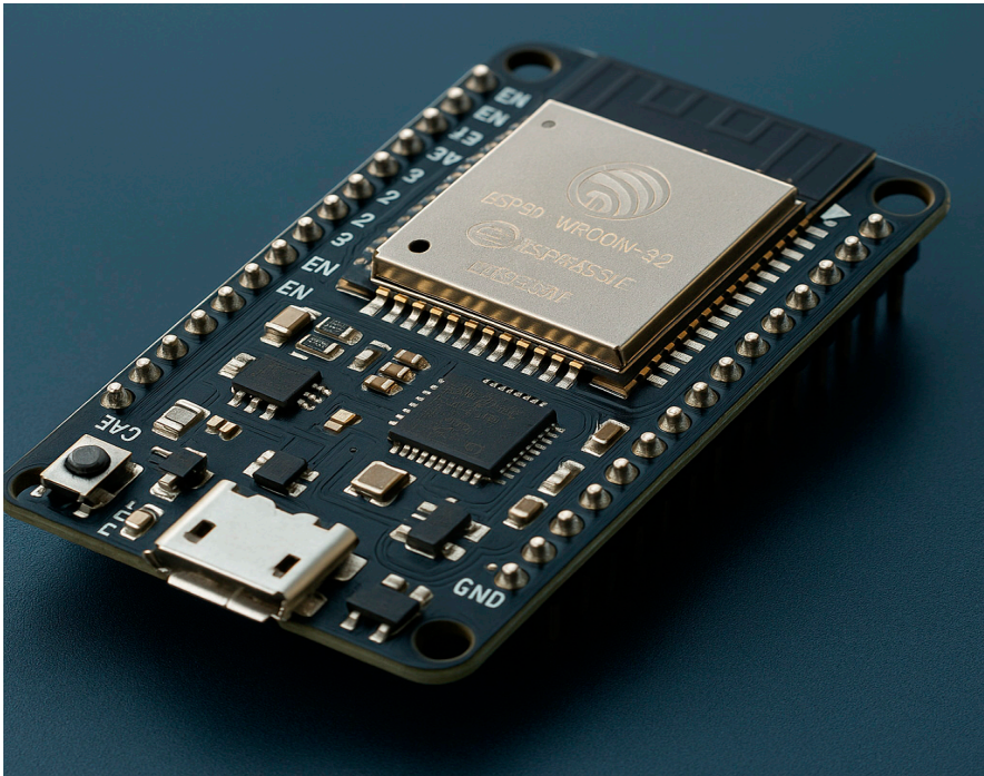
Figure 1. ESP32-WROOM-32 development board, highlighting its compact layout, robust microcontroller chip, and micro-USB interface.
