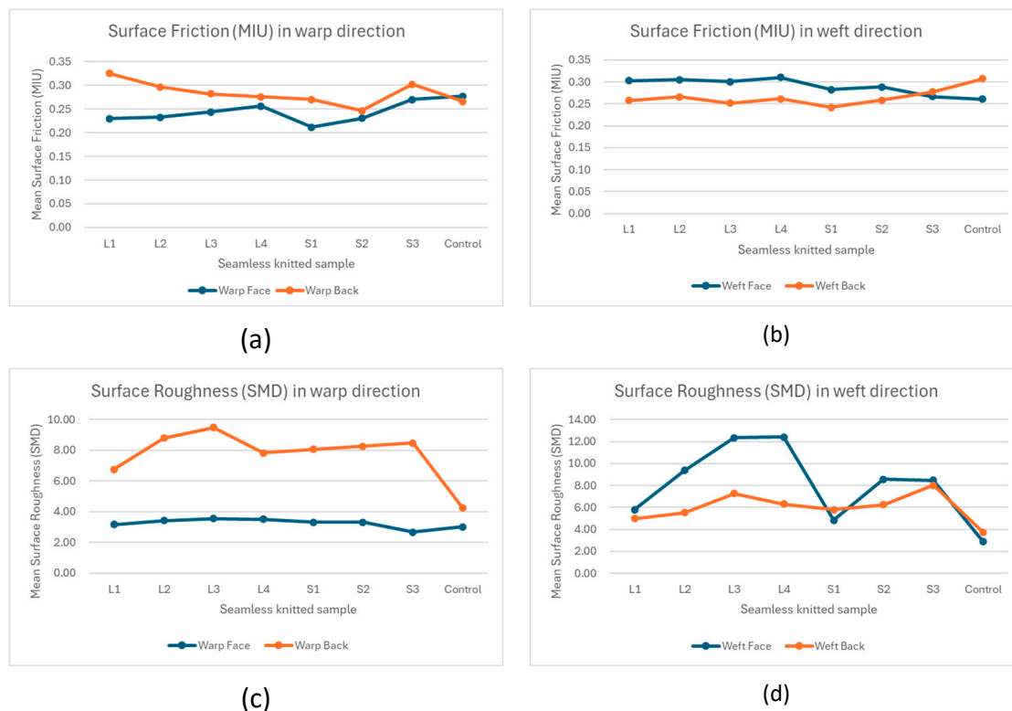
Figure 8. Surface friction (MIU) of seamless punch lace knitted fabrics and the control fabric in (a) warp and (b) weft direction; surface roughness (SMD) of seamless punch lace knitted fabrics and the control fabric in (c) warp and (d) weft direction.
