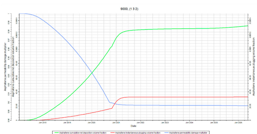
Figure 21. Deposition, Permeability, and Plugging at Injector. This figure shows all three outputs evaluated for this study at the injector in layer 2.
