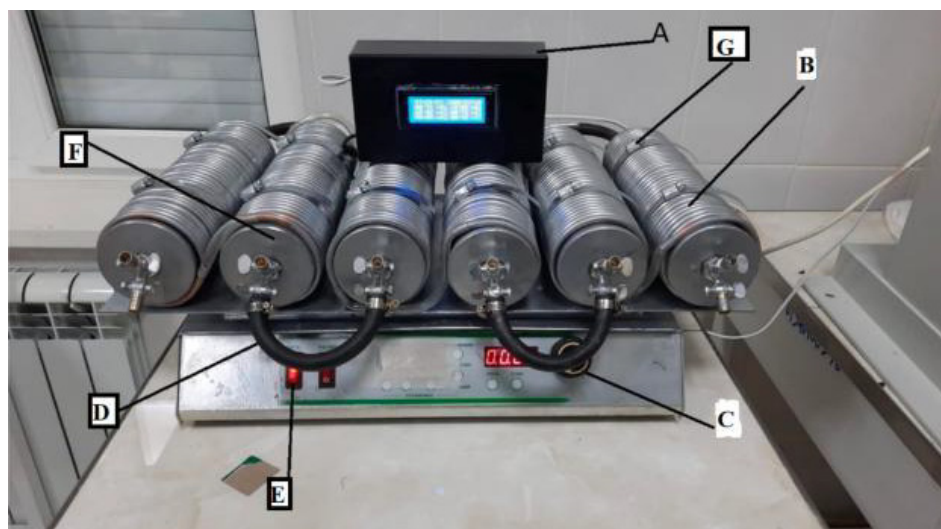
Figure 1. General view of the reactor, where A—information processing receiver with temperature control system at each stage; B—copper line of the heating/cooling system with outputs for connection to Hubert furnaces; C—adjustment of the horizontal movements speed of the reactor base, next to it a display showing the number of movements per minute the platform makes based on a motion sensor; D—reactor on/off button, next to it the on/off button plug for the autonomous heating and cooling system; E—carbon fiber hose for connecting reactor stages to each other, providing 6 mixing stages in the reactor; F—reactor pipes (stages) with an advanced design of reactor lids; G—holders for reactor pipes (stages).
