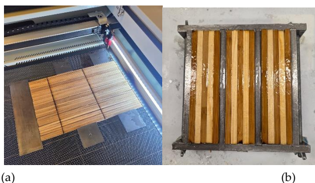
Figure 1. Specimen preparation: a) laser cutting of Moso bamboo strips to the required dimensions; b) application of adhesive to bamboo and timber strips, and assembly in the mould.
