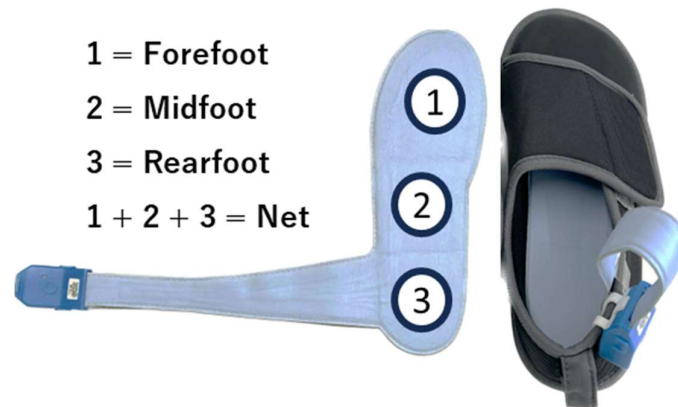
Figure 1. Overview of the 3-sensor plantar force measurement insole device. Three sensors are inserted in a 3-mm-thick shoe insole. The insole is inserted in a commercial Velcro shoe, and the data acquisition unit is fixed using an attached clip on the shoe.
