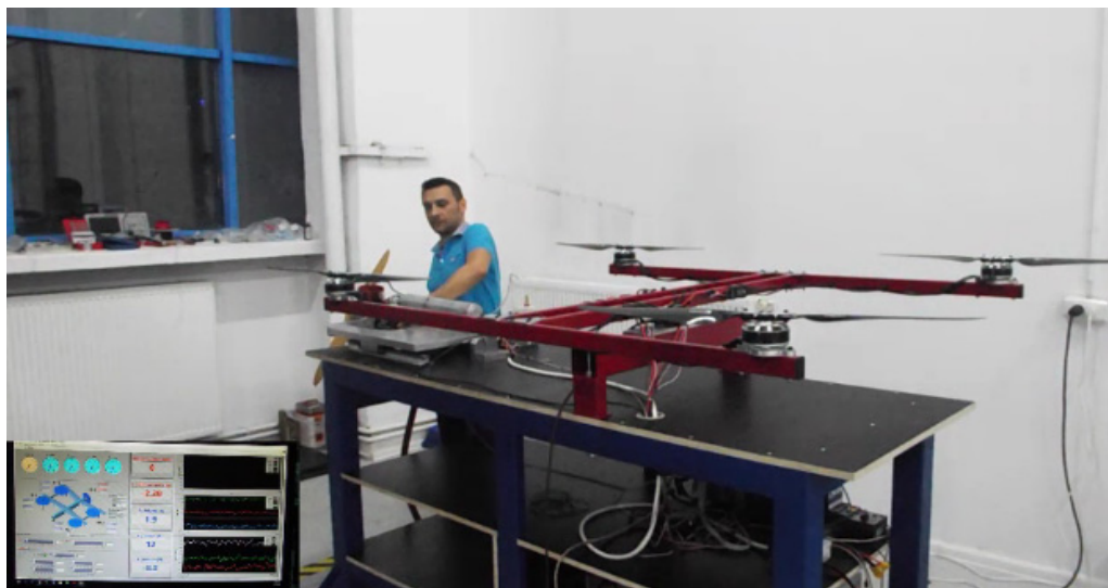
Figure 18. Laboratory testing of the VTOL system (ground testing).
