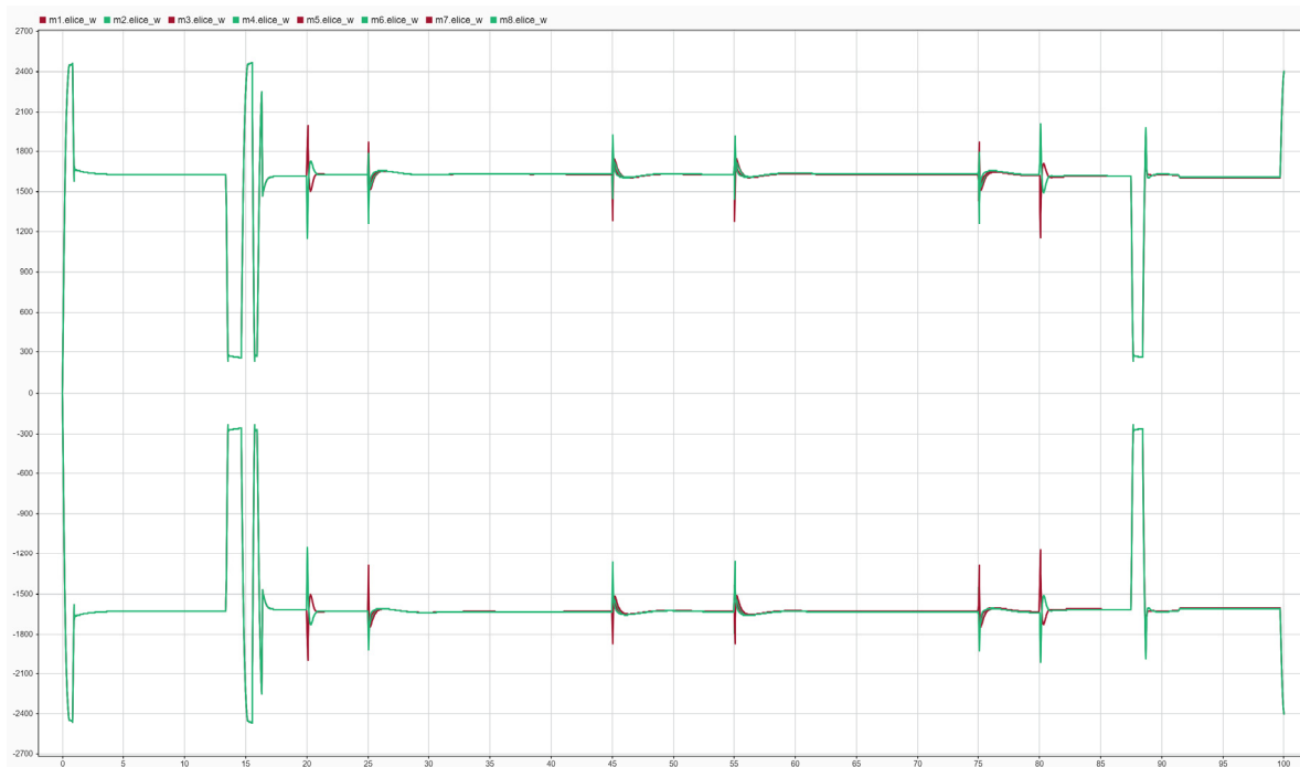
Figure 13. Time evolution of the rotational speeds (RPM) of the propulsion units.
