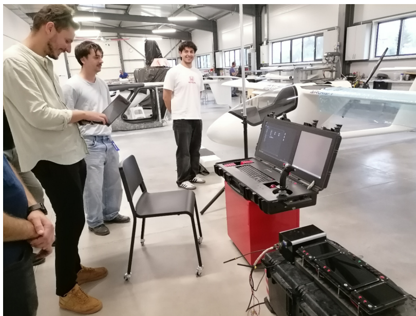
Figure 23. Intermediate stages of preparation for the initial flight tests, focusing on the configuration and integration of the communication subsystem and the Ground Control Station (GCS) at the AVI Aircraft manufacturing and test facility.
