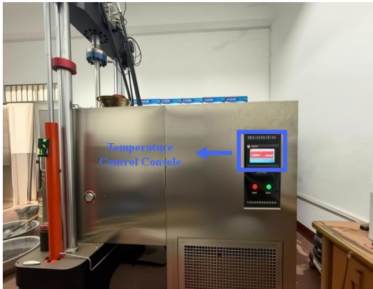
Figure 2. Servo-Hydraulic Dynamic Test System with Environmental Chamber.
