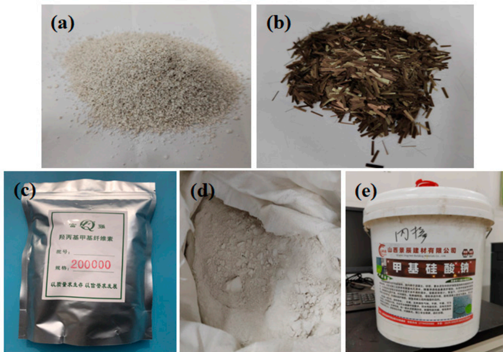
Figure 2. Raw materials, (a) vitriified microbeads, (b) basalt fiber, (c) HPMC, (d) calcium hydroxide, (e) sodium methylsilicate solution.
