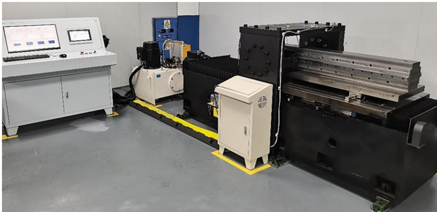
Figure 16. Multi-parameter test bench for rolling linear guide pairs.
