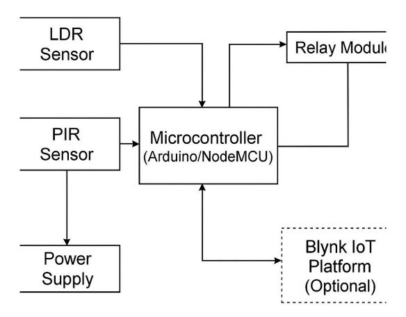
Figure 1. Block diagram of the IoT-based smart street lighting system.
