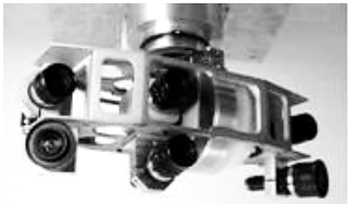
Figure 6. Camera set used in VaMoRs in the AutoNav-project 1997 – 2003.
