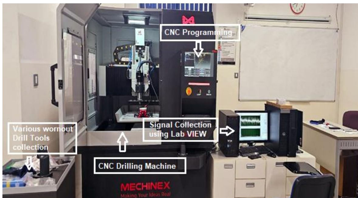
Figure 2. Signal collection from the CNC drilling machine.
