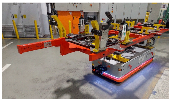
Figure 6. Photograph of the prototype FTPD mounted on an automated guided vehicle.
