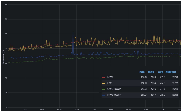
Figure 3. The dashboard displays root zone temperatures in different cooling treatments.
