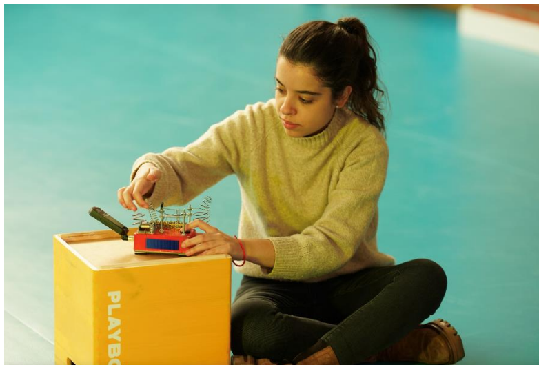
Figure 4. Play Box connected to a wireless sound system. The signal is transmitted to a sound card via a commercial plug&play 2.4GHz wireless audio transmission device. .
