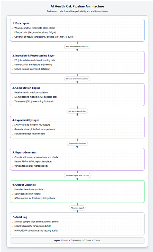
Figure 2. Data Flow and Report Generation Process: pipeline from inputs and ETL through anomaly detection, forecasting, SHAP explainability, and report/audit outputs.
