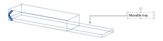
Figure 2. Service gateway and hopper of vertical fruit showcase.
