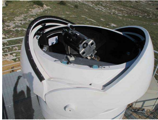
Figure 6. GDIMM instrument at Calern Observatory [53].
