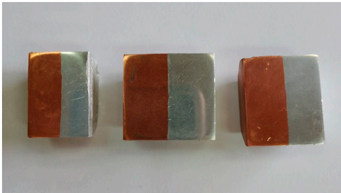
Figure 6. Al-Cu joint samples for microstructural investigations. Friction times (left to right: 6.5, 7.5, 9.5 s).
