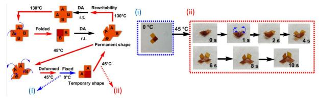
Figure 4. Preparation of sample for shape memory test and shape transformation of PFSLA/M<sub>2</sub>-6/1 with rewritable functionality.
