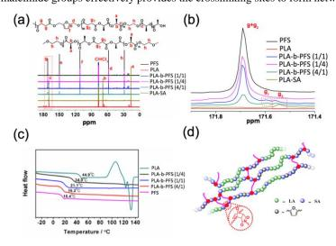
**Figure 1.** (a) <sup>13</sup>C NMR spectra of PFS, PLA and PLA-*b*-PFS polymers and (b) its magnified spectra at the region of 171.4-171.9 ppm. (c) DSC curves of PLA, PFS and PLA-*b*-PFS with different molar ratio of LA to FS and (d) a schematic illustration of PLA-*b*-PFS crosslinked by M<sub>2</sub> through DA reaction.
