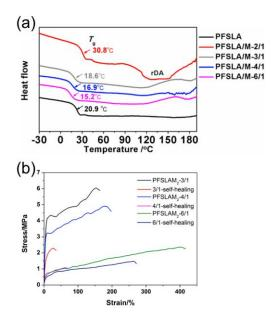
**Figure 2**. (a) DSC curves of PLA-*b*-PFS/M<sub>2</sub> with different crosslinking density and (b) comparison of stress-strain curves for PFS-b-PLA/M<sub>2</sub> at various crosslinking density and its self-healed (after 5 days) analogs.
