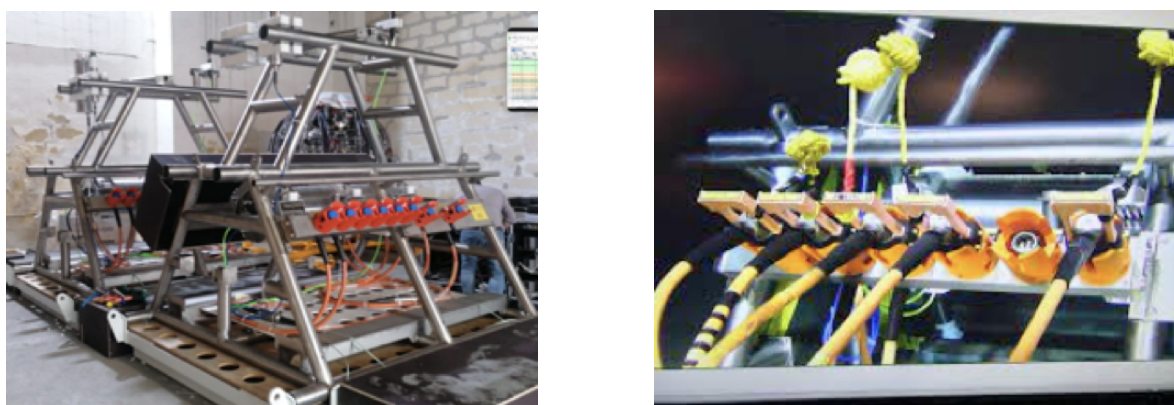
Figure 2. Picture of two Junction Boxes subsea assets in the assembly hall (on the left ), and during the deployment campaign on the seafloor of the Portopalo site after the connection with the observatories ( right ).
