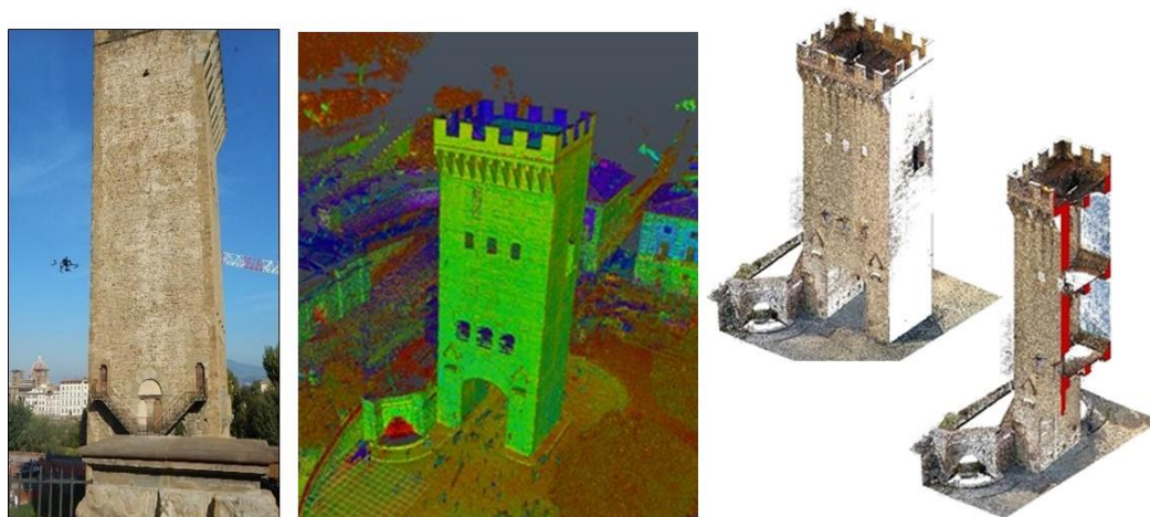
Figure 3. From left: drone photogrammetric survey, point-cloud restitution, H-BIM model (elaboration A.L. Ciuffreda).
