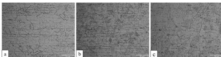
Figure 2. Optical microscope images of samples a) annealed, b) after the ECAP, and c) after the ECAP-recovery treatment.
