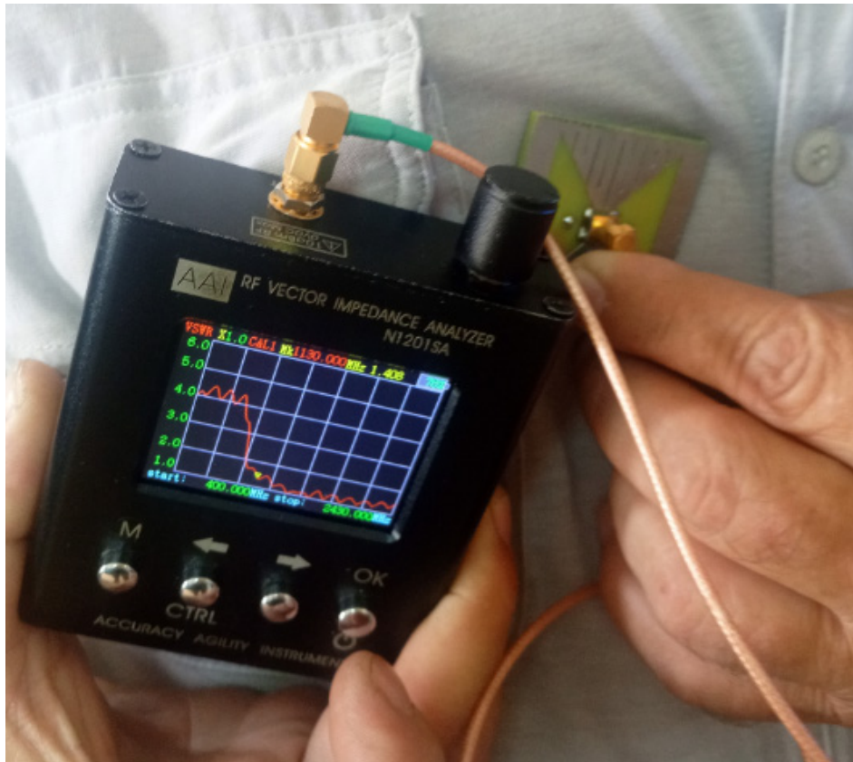
Figure 3. Broadband antenna during SWR measurements.
