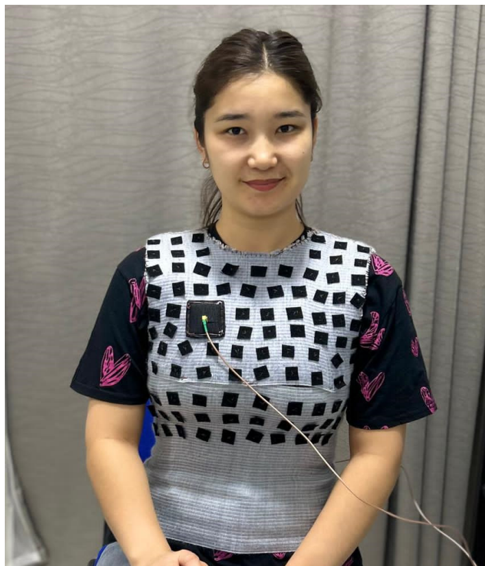
Figure 5. Attachment of antennas to the human body using an elastic vest and Velcro fasteners.
