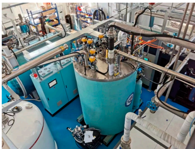
Figure 8. 80 L/h helium liquefier for the superconducting magnet test platform.
