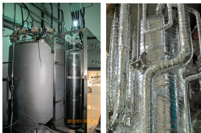
Figure 5. Cold box of 40 L/h helium liquefier and the internal photo.
