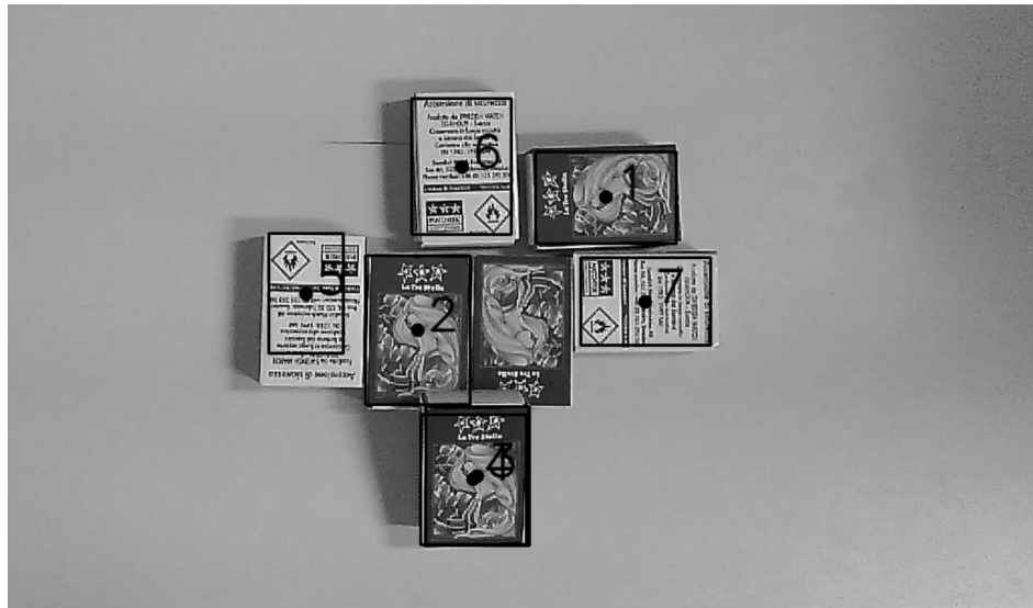
Figure 4. Detection of SIFT technique tested on matches boxes.
