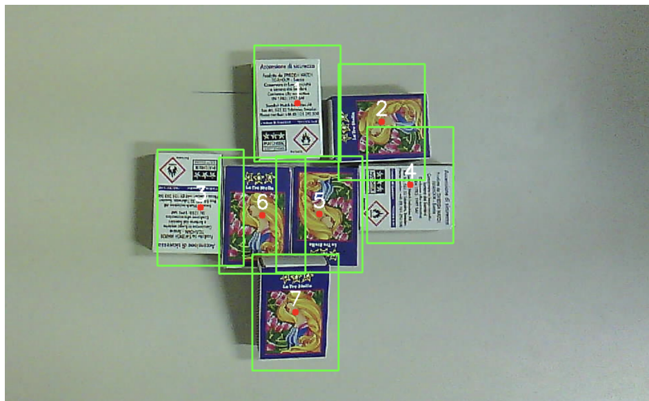
Figure 6. Detection of Haar Classifier technique tested on matches boxes.
