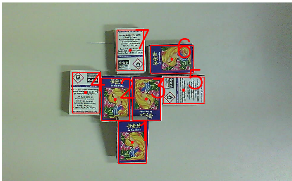
Figure 3. Detection of Pattern Matching technique tested on matches boxes.
