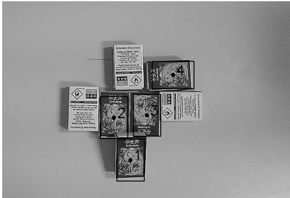
Figure 5. Detection of ORB technique tested on matches boxes.
