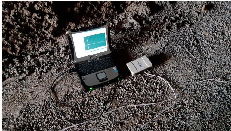
Figure 8. The rugged PC used for the field test and the NI-DAQ card used for the data acquisition.
