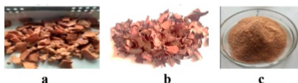
Figure 4. Intermediate (b - after drying) and final (c-after drying and grinding) conversion products of the solid insoluble residue of the peel (a).
