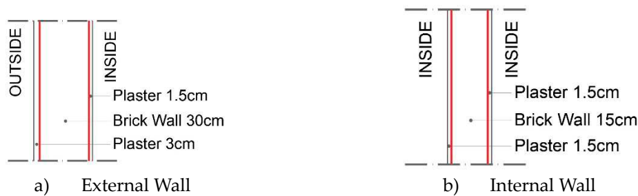
Figure 6. Existing building exterior and interior wall section.
