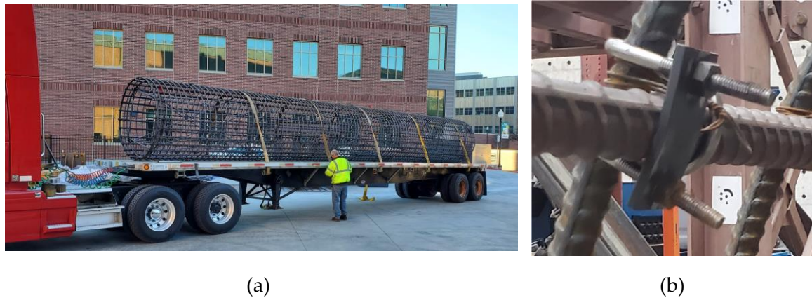
Figure 8. (a) Transportation of the cage specimens prior to testing, (b) bending of the plates in a tight-fit connection.
