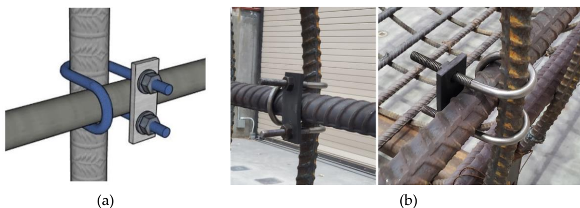
Figure 1. (a) Schematic view of Cage Clamp connection, (b) an assembled Cage Clamp connector for a cross-bar connection in a rebar cage.
