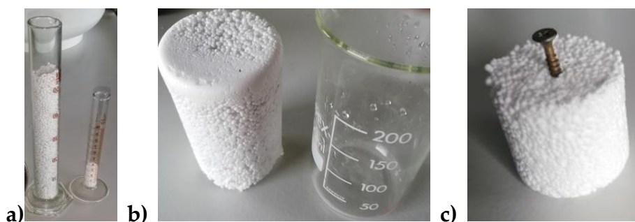
Figure 14. Volume occupied by EPS beads before and after the MW-assisted heating.
