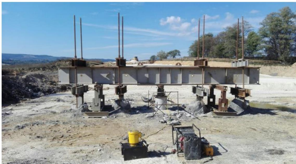
Figure 1. Using tension piles as reaction piles for static loading tests (Rainer, 2019).
