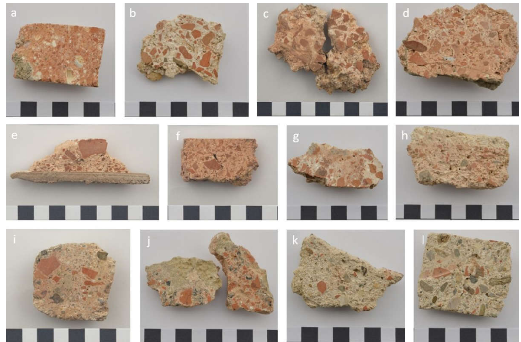
Figure 1. “Brick” mortars from Viminacium (dating from the 2 nd to the 6 th century): a. principium floor; b. city baths floor; c. city baths plaster; d. city baths floor; e. city baths plaster; f. city baths plaster; g. city baths plaster; h. tomb plaster; i. sarcophagus base; j. villa floor; k. villa bedding mortar; l. early Byzantine rampart bedding mortar. Photo-documentation of the MoDeCo2000 project.
