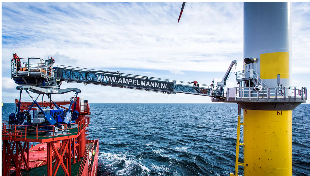
Figure 2. Stewart platform-based motion compensated gangway. (Courtesy of Ampelmann).
