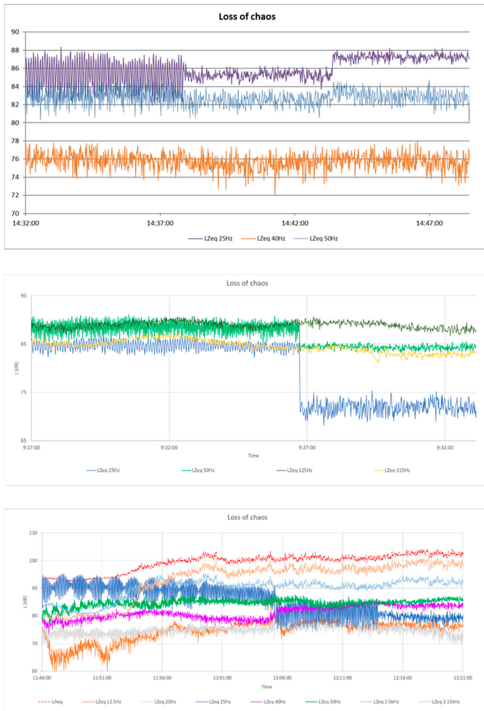
Figures 6, 7 and 8. Loss of chaos in different third-octave bands during the installation of thermoacoustic instability episodes. Graphs from the environmental sound pressure meter in the engines room. The tests according to ISO 3744 [23] were carried out during these measurements (only one engine in operation). Please note the ordered pattern before the jump in the sound pressure levels in the considered band.
