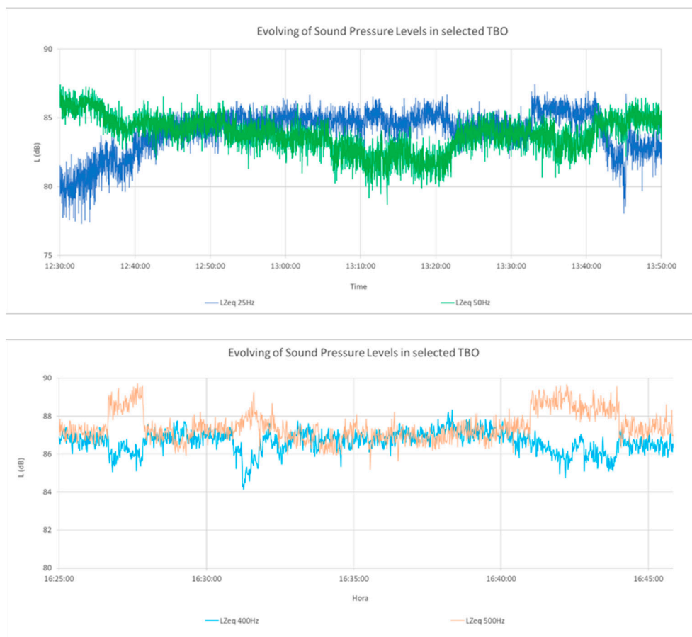
Figure 4. Sound pressure levels in selected third-octave bands during steady running of the engines.
