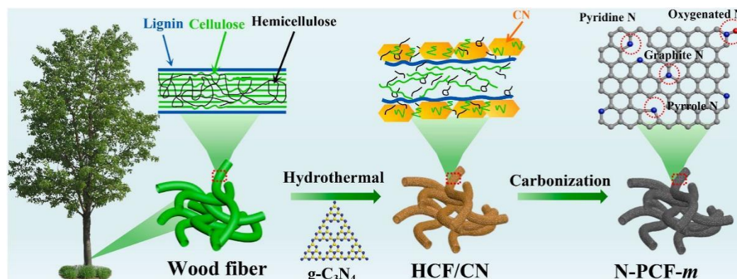
Figure 1. Schematic diagram of the synthetic procedure for N-PCF-m. Reprinted with permission from Ref [39], Copyright 2022 Elsevier.
