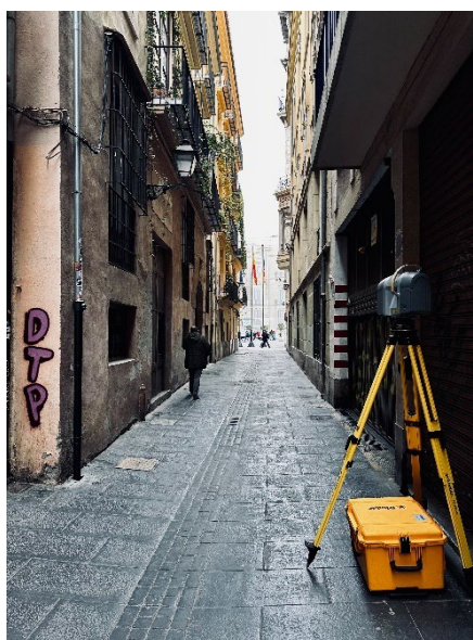
Figure 1. Trimble TX6 equipment installed to lift the façade of the Palacio Más. Source: Own authorship.
