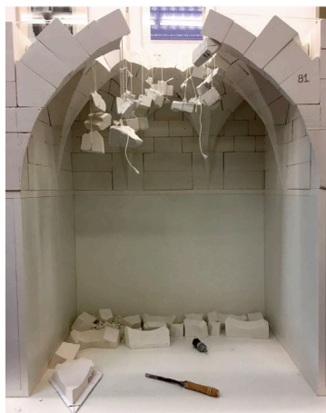
Figure 11. Navarro's hypothesis on how to complete the vault. Photo: Pablo Navarro Camallonga.
