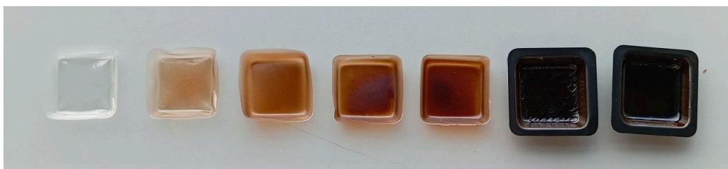
Figure 4. The visual appearance of PVA/BSF proteins films in % w/w 100/0, 90/10, 70/30, 50/50, 30/70, 10/90 and 0/100 from left to right.
