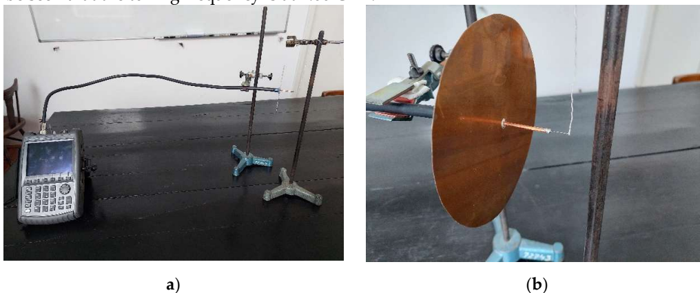
Figure 8. Pictures of the experimental arrangement for proving the microwave dielectrophoresis force: general view (a) and details with the antenna and pendulum (b).
