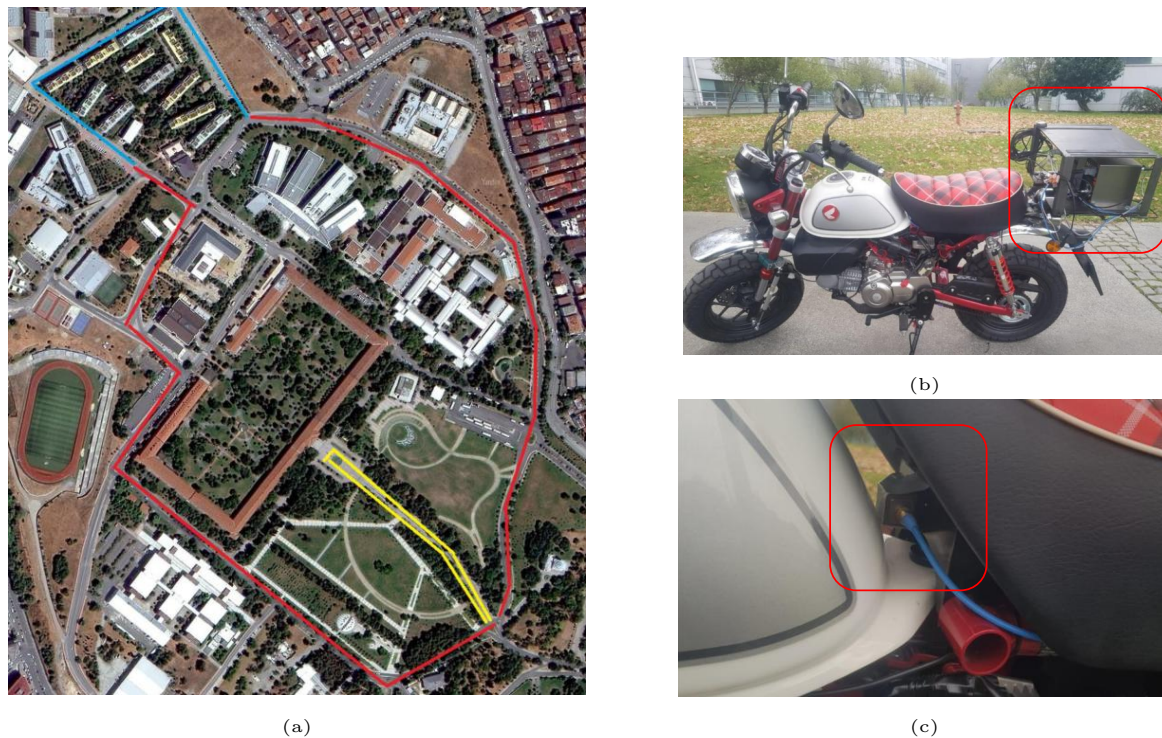
Figure 2. Overview of the data acquisition system and test track: (a) the test area in Yıldız Technical University, (b) the motorcycle equipped with the measurement unit, (c) close-up view of the acceleration sensor placement.
