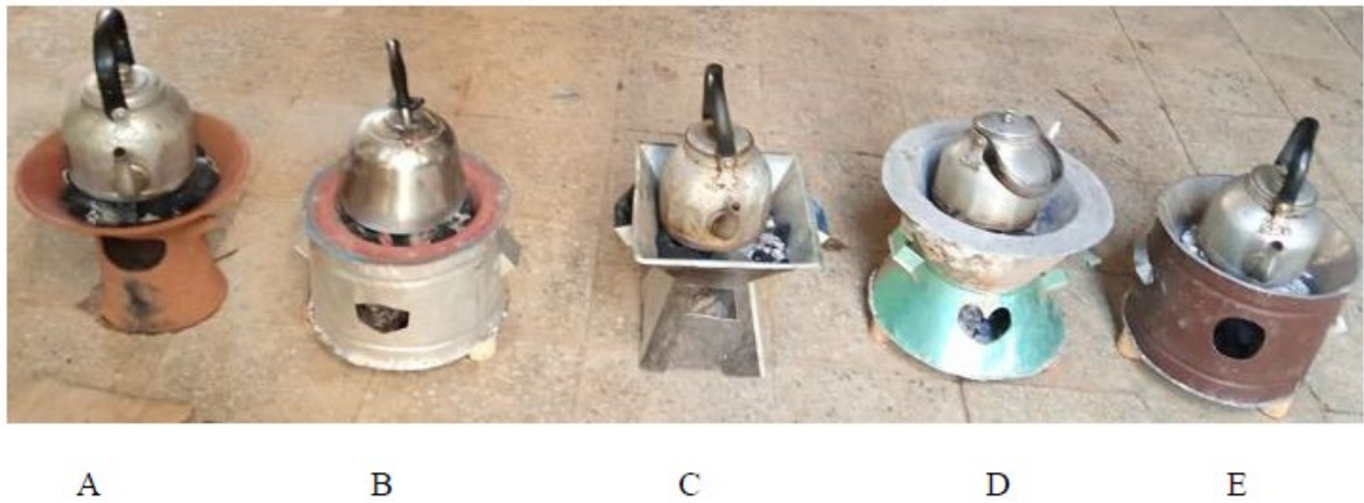
Figure 2. Stove Types Selected from the District. Type 1 (clay stove), B) Type 2 (cylinder stove Insulated with clay), C) Type 3 (Rocket stove without insulation), D) Type 4 (Rocket stove with insulation), E) Type 5 (Cylindrical stove without insulation).
