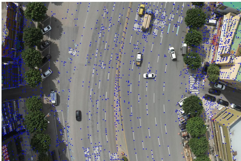
Figure 11. 3D position information associated with input image keypoints (blue dots) is based on the reference model.
