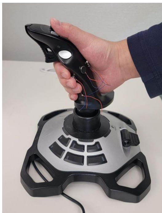
Figure 3. Logitech Extreme 3D Pro Joystick with Tactors Attached to Provide Vibrational Feedback.
