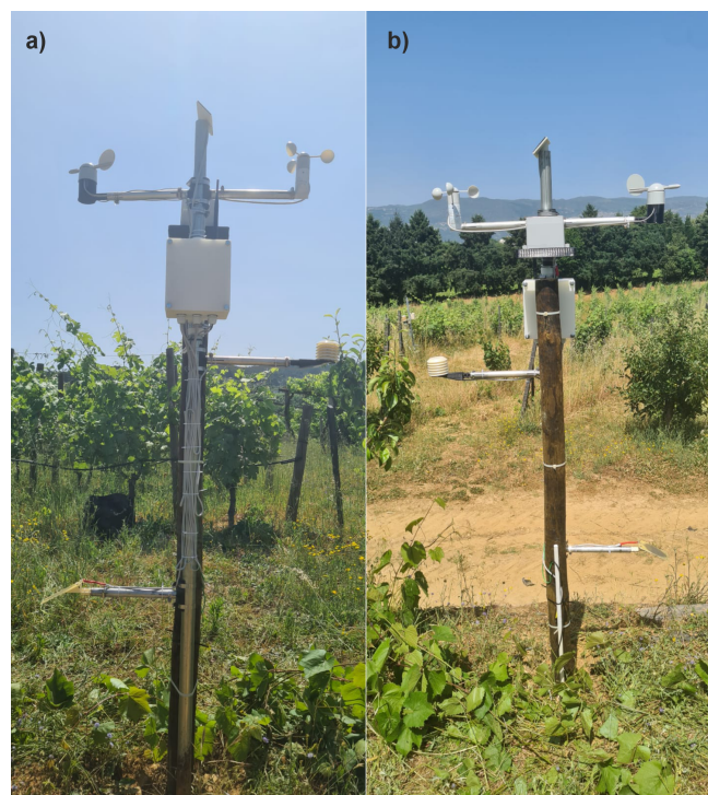
Figure 5. Deployed field prototype in the vineyard. (a) Front view of the complete station; (b) back view showing sensor mounts and enclosure placement.
