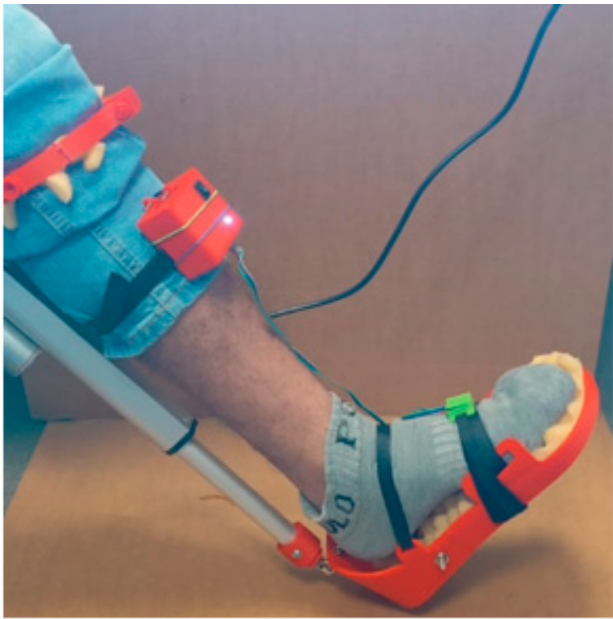
Figure 20. Snapshot of a second functional test of ankle joint movement dorsal and plantar flexion.
