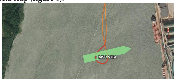
Figure 6. Trajectory of the POST PANAMAX container vessel during turning in port ships turning basin (T/H about 0.95) received by calibrated simulator and on the real ship.
